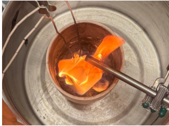
Figure 11. Picture taken during the open burning of the plastic mulch film. The brown wires are the thermocouple for monitoring the burning temperature, and the stainless tube is the sampling inlet for air pollutant monitoring.
