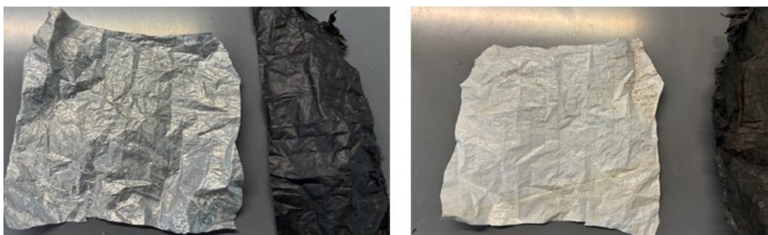
Figure 5. Plastic mulch films examined in furnace experiments: white/aluminized polyethylene and black polyethylene.
